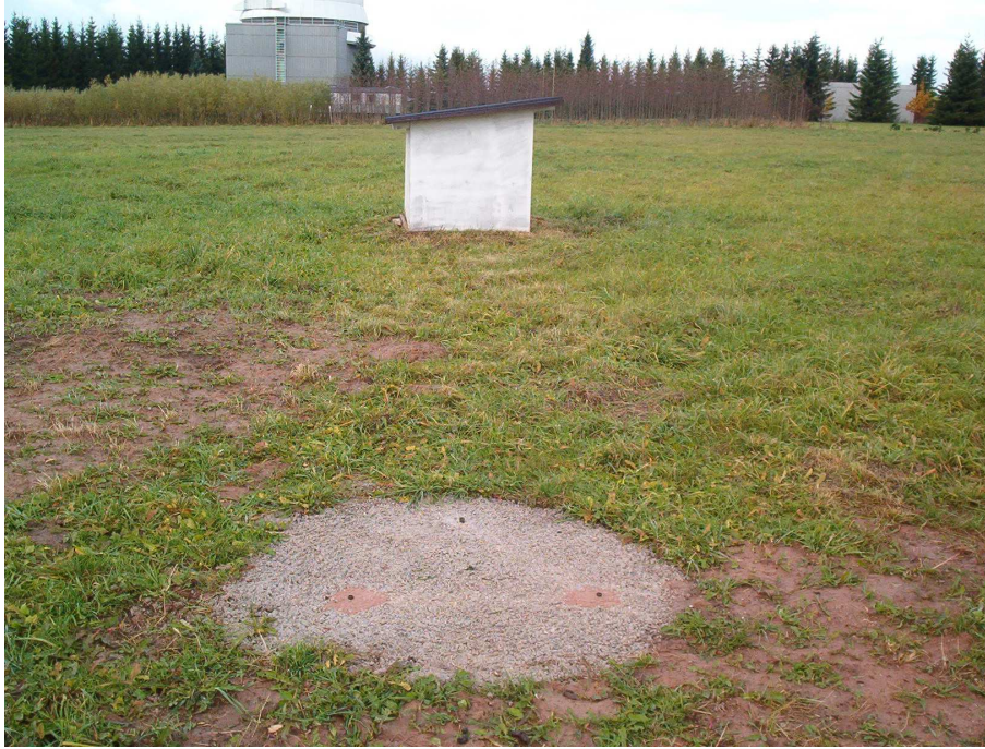
Figure 3: The magnetometer hut and the concrete basement for absolute measurements at the Tartu station.
